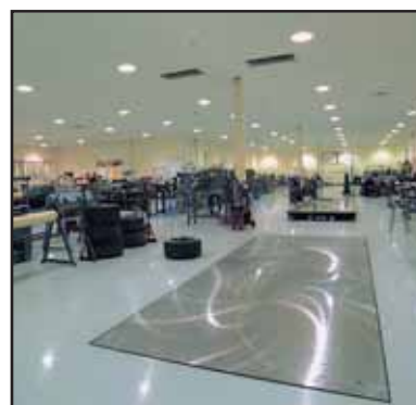
A set-up plate, the last station a car visits before going to the race track.
